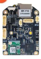
MY-Y10 is a 3MP Dual Band WiFi PTZ IPC module designed for indoor home surveillance environments or smart robotics applications. With its advanced features, it provides reliable monitoring and control, making it an ideal choice for enhancing security and automation in your home.
